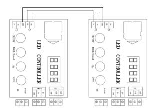
TTL: single-and two-wire signal interface.
