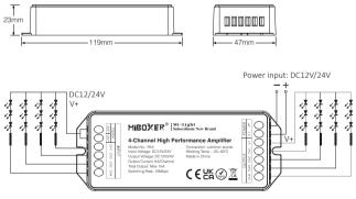
Attention: 1. LED strip must be DC12V or 24V. 2. Output and input voltage must be the same.
